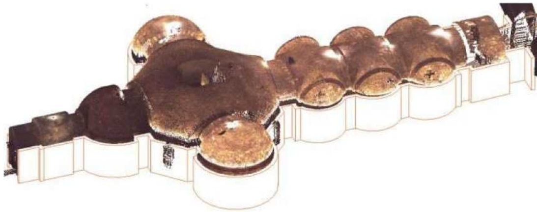
Figure 4. Tomb point cloud represented in Revit Environment.
